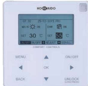
HEATING + DHW operating mode
